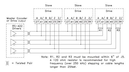
Figure 29: Master/Slave Encoder Connections
